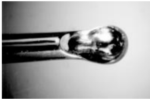
Figure 1 The tip of the 'gonioscraper'. The bowl is 300 \mu\text{m} in diameter with its edges sharpened.
