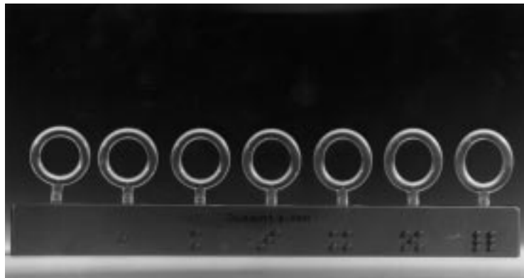
Figure 1 The keratoscopic astigmatic ruler consists of a rack of lenses—a circular lens and six increasingly elliptical lenses for 1 to 6 dioptres of astigmatism. Each keratoscopic lens works like a Maddox rod producing a bright aerial image of the microscope's light that is reflected back to the observer by the corneal surface. The metal handle has raised marks to enable the user to determine, by palpation, the lens in use when at the microscope. The circular lens is used for the initial assessment of the astigmatism and to align the handle of the KAR with the long axis of the elliptical image. The correct distance which hold the KAR from the eye is determined by observing the whole limbal diameter just within the short internal diameter of the lens (the "sight"). Once aligned the image is observed with each lens in front of the cornea, the measurement end point is when the image appears most circular. Past the end point the image becomes elliptical perpendicular to the handle.
