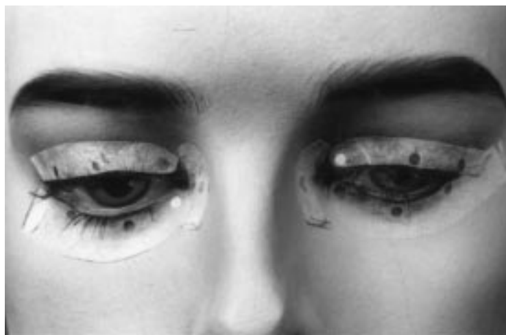
Figure 2 Dosimeters in place on the manikin's eyelids.
