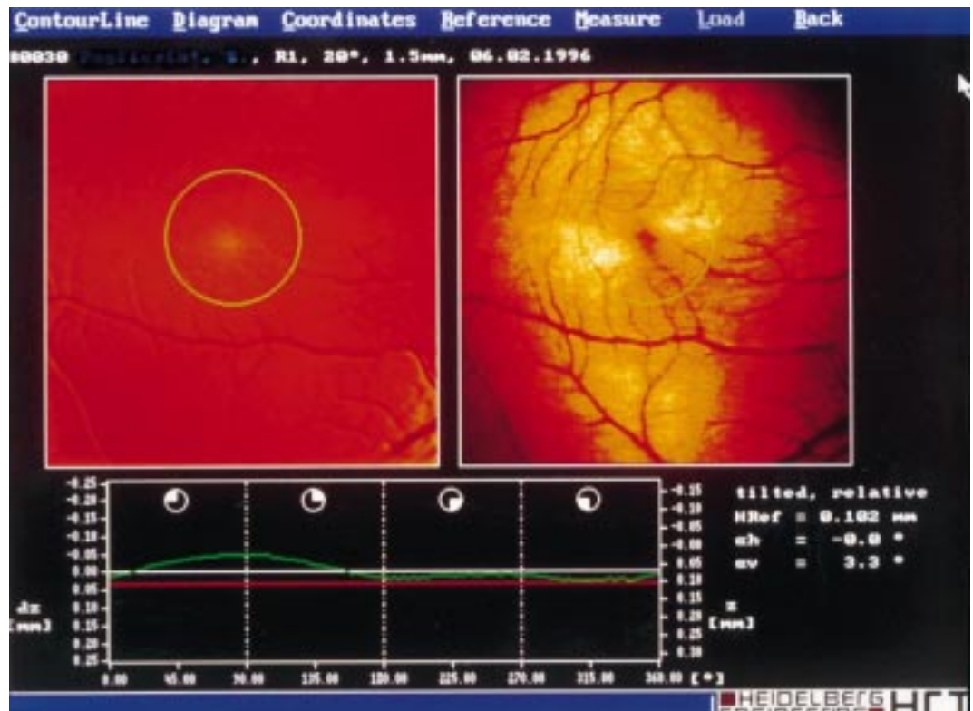
Figure 1 HRT scan of a normal macula in a healthy 36 year old man. The height variation of the contour line is shown in green and the reference plane (in red) is adjusted to the lowest point of the contour line. The scan is centred at the fovea. The circle centre is the fovea, the diameter is 2 mm. The scale (25 mm) is given on the left hand vertical axis.
