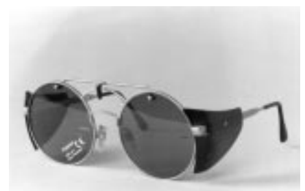
Figure 2 Spectacles with variable polarisation used to explore the effect of polarisation at different axes.
