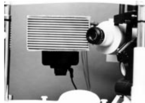
Figure 1 Front view of the photographic system, consisting of the target and a Brown macrocamera.
