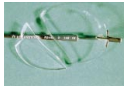
Figure 3 The frameless spectacles; fractured by a low velocity accident.
