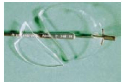
Figure 3 The frameless spectacles; fractured by a low velocity accident.
