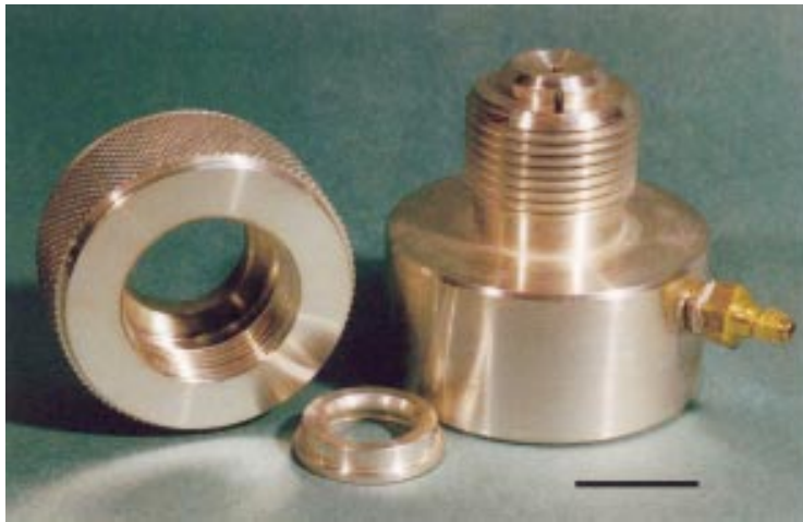
Figure 5 An artificial anterior chamber designed to mount cadaveric porcine corneoscleral buttons.
