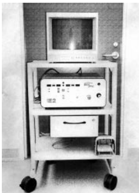
Figure 1 Endoscopic cyclophotocoagulation laser unit. The laser console is compact and the high resolution monitor is used to guide the laser probe for direct, selective treatment of ciliary processes.
