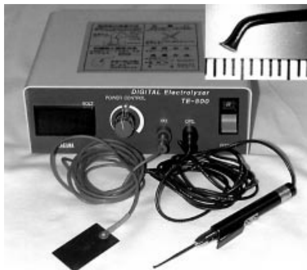
Figure 1 Digital electrolyser and a flat electrode for corneal electrolysis (inset, one division is 1mm).
