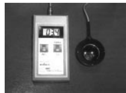
Figure 1 Photograph showing the Goldmann contact lens with a pressure sensor mounted into the holding ring of the contact lens and connected to a display.
