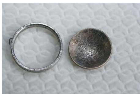
Figure 2 Picture of actual Sr-90 applicator with perforated stainless steel ring to fix the applicator to the sclera.
