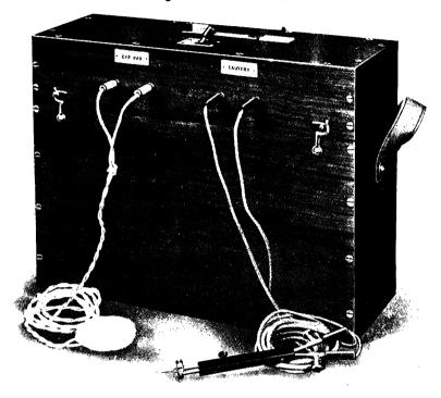
THIS method of heating an eye pad is perfectly safe as it forms a unit independent of the ordinary high-voltage house supply, and removes any possibility of shock to the patient or operator should a wire become exposed. In addition to the heating pad, there is provision for a cautery needle.
