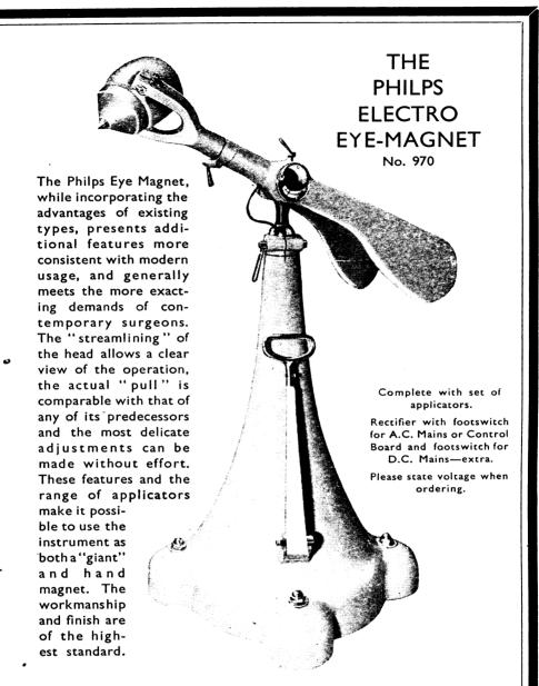
Operating Theatre regulations require flameproof switch gear to be used with all apparatus of this type. Where A.C. only is available a Rectifier is necessary. This can be supplied complete with suitable footswitch at extra cost.
