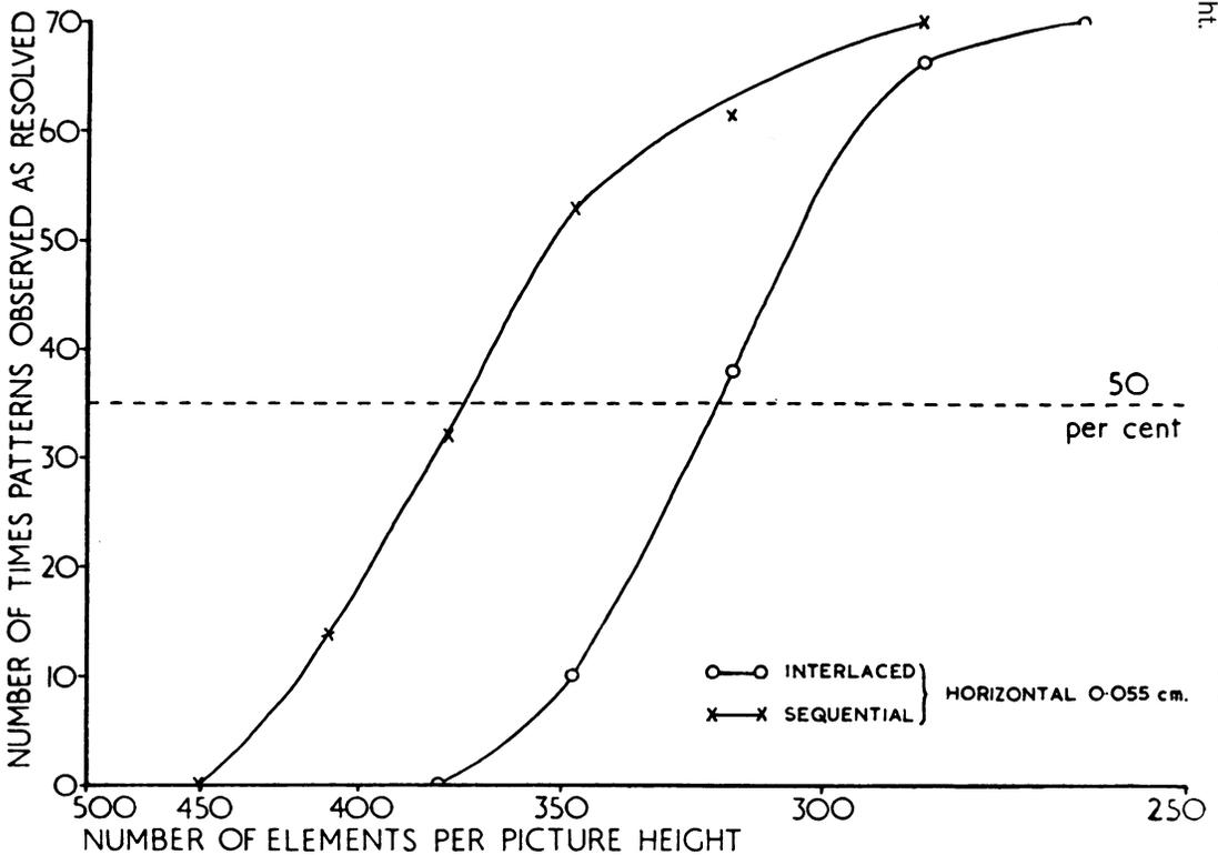
FIG. 4.—Vertical resolution of Cobb-Moss test pattern by variable definition channel.
