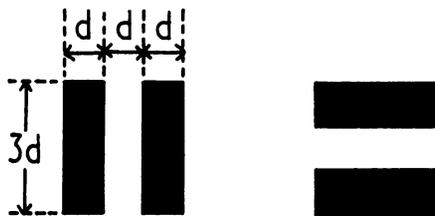
FIG. 3.—Cobb-Moss test pattern for testing vertical and horizontal resolution.
