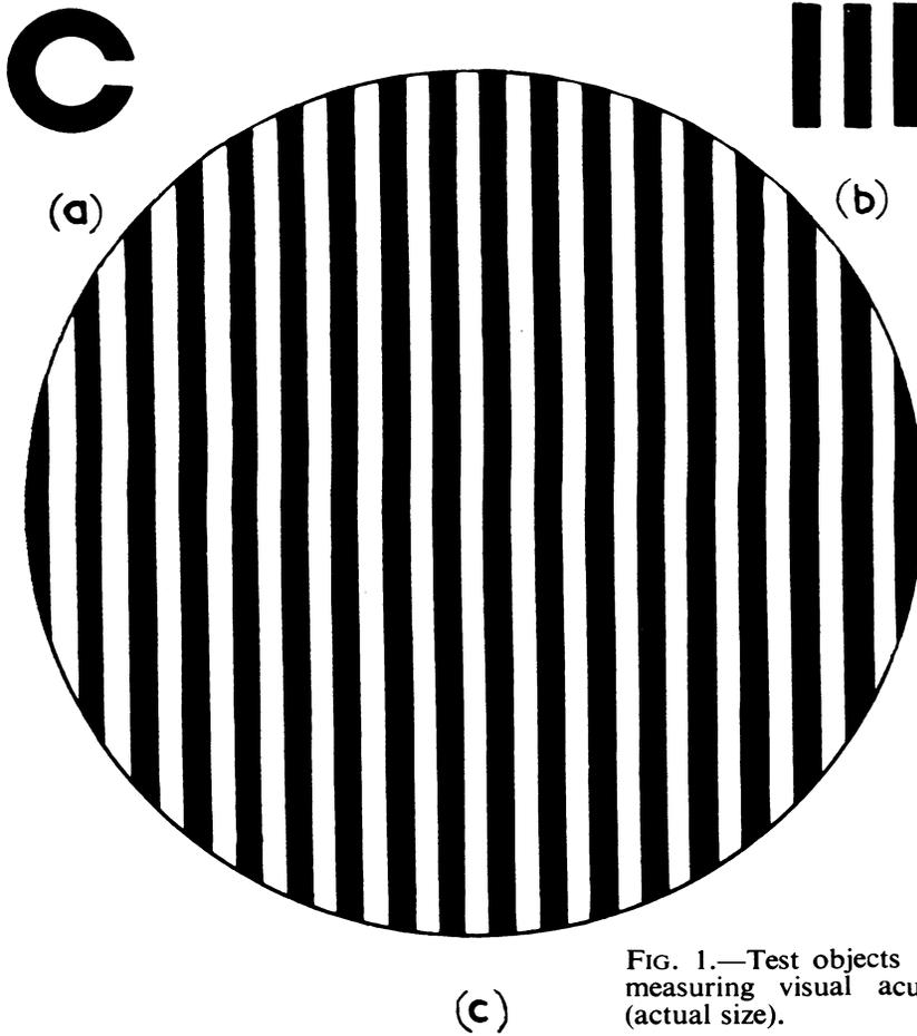
FIG. 1.—Test objects for measuring visual acuity (actual size).
