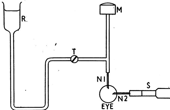
FIG. 1.—Diagram of apparatus for determination of ocular distensibility by manometric method.
