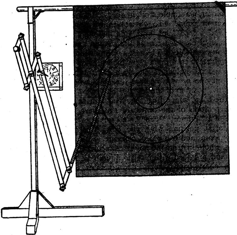
pushing the rod horizontally through the hole in the standard, or by twisting it in the manner of a roller blind, the position of the curtain (and fixation object) may be adjusted to the rest of the instrument. Attached to the standard, 4 feet from the floor and on the same side as the curtain, a board holds the chart by means of suitable slots into which the chart is slipped into position.
