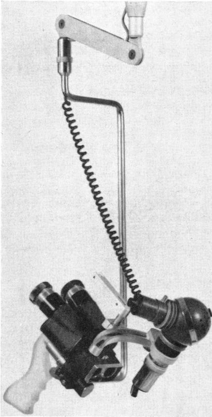
FIG. 5.—Independently suspended gonioscope may be released at any desired angle of observation. The position of the instrument is exactly retained.
