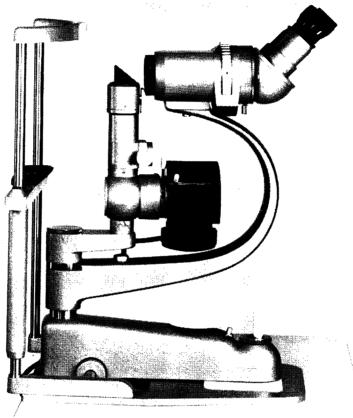
For the first time in slit-lamp microscopy the ophthalmologist has the advantage of the versatility and convenience of a pancratic zoom optical system. Simply by rotating a control a continuous magnification of 7x to 40x is obtained.
