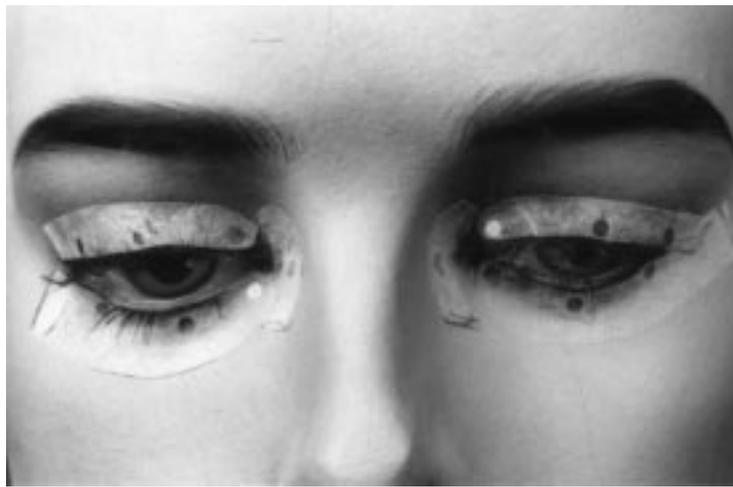
Figure 2 Dosimeters in place on the manikin's eyelids.
