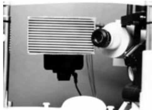
Figure 1 Front view of the photographic system, consisting of the target and a Brown macrocamera.
