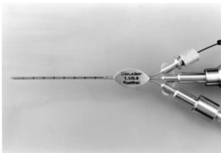
Figure 2 The modified Bowman probe (Geuder) with 1.1 mm outer and 0.9 mm inner diameter. At the upper end the connection for the endoscope, in the centre the laser fibre and at the third opening the syringe may be attached. The marks in a range of 5 mm are clearly detectable.
