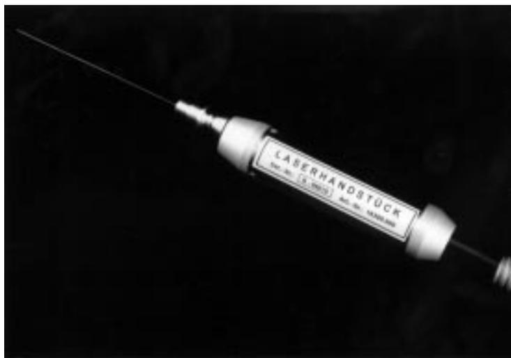
Figure 1 The laser hand piece (Schwind) with the fixed sapphire laser fibre of 350 µm.
