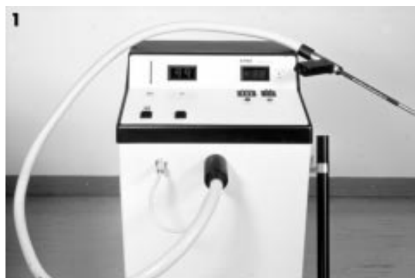
Figure 1 Cryosurgical equipment Erbokryo PS (made by Erbe Elektromedizin GmbH, Tuebingen, Germany) for liquid nitrogen cryosurgery, used for treatment of the first series (1979–88). The equipment was connected to pistol handle and contact probe by a relatively thick, vacuum insulated flexible tube.
