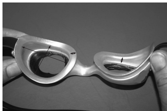
Figure 2 Photograph of goggles with arrows illustrating the vertical width, horizontal width and rubber seal width on the left goggle side, with rubber seal depth on the right.
