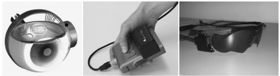
Figure 1 A schematic illustration showing the surgically implanted stimulating microelectrode array, and inductive coil telemetry link of the Argus II system (left). The external portions of the system consist of a video processing unit (VPU) (middle) and a miniature camera mounted on a pair of glasses (right).
